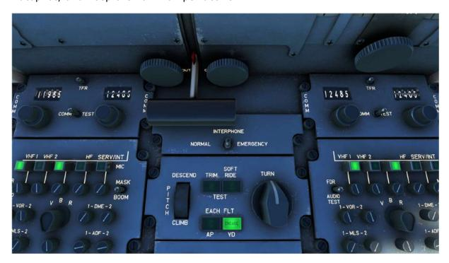
If only the YD Button is lit, the Yaw Damper can be turned off by pressing the lit YD Button. The Yaw Damper cannot be turned off when the Autopilot is active.
