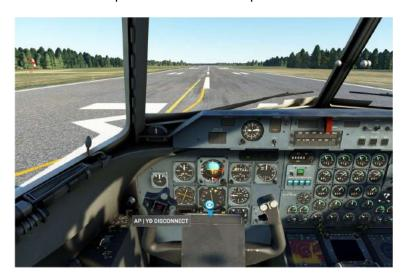
A quick left-click on the Red Button will disengage ONLY the Autopilot, left-clicking and briefly holding the left-mouse button will disconnect BOTH the Autopilot and the Yaw Damper at the same time.
