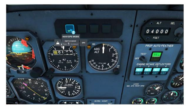
The GPS units feature a function that mirrors this, selecting VLOC on the GPS unit is essentially the same as pushing the NAV | GPS button shown above.
