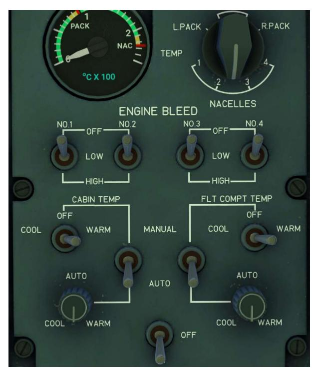
1. Check that all four Engine Bleed Switches are in the OFF position.
