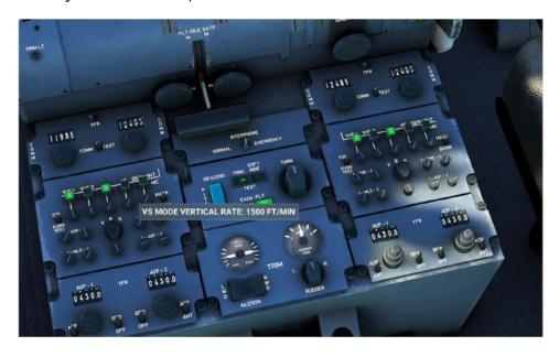
If you have ToolTips activated, your VS Mode Vertical Rate will be indicated as shown above, and will change as you move the mouse wheel up or down.
