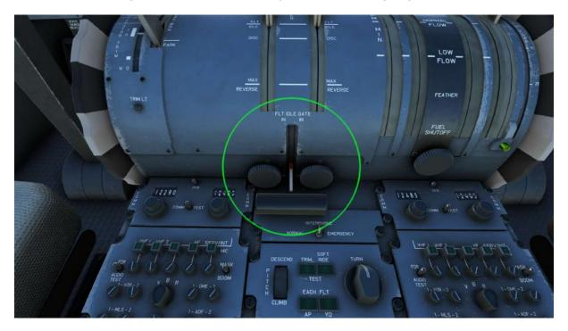
It is automatically triggered by the wheels leaving the ground at take-off, the wheels touching the ground upon landing. The Flight Idle Gate snapping open or shut produces an odd clunking sound that can be heard very distinctly from within the cockpit.
