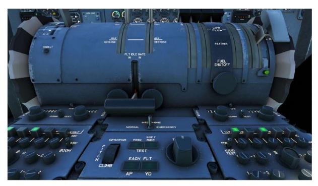
Switching on the Autopilot will automatically also switch on the Yaw Damper, and both the AP and YD Buttons will light up to indicate that they are active:
