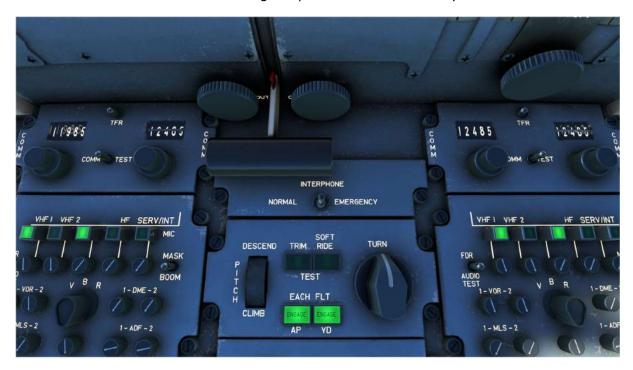
Should you wish to only engage the Yaw Damper, you may either press the YD Button when both the Autopilot and Yaw Damper are off and both the AP and YD Buttons are unlit, or push the lit AP Button once again, as this will turn off the Autopilot, and keep the Yaw Damper active:
