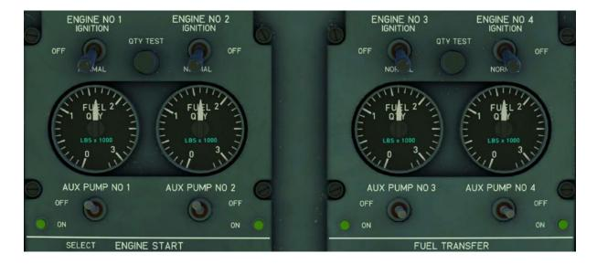
1. Check that all four Engine Ignition Switches are in the NORMAL position.
